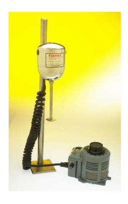
Fann Laboratory Mixers are two speed mixers, available in both 115 and 230 volt models. No load test speeds of 11,000 and 15,000 rpm. Supplied with the standard impeller blade for mixing either water-base or oil-base drilling fluids. Powerstat<sup>®</sup> variable transformers (sold separately) are used to provide an extended mixing speed range.
